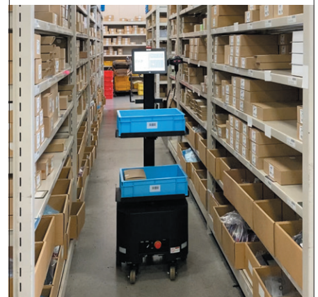
Figure 1 Rapyuta PA-AMR collaborative picking assist robot of Rapyuta Robotics operating in the Heiwajima Logistics Center of Nippon Express (provided by Rapyuta Robotics)
