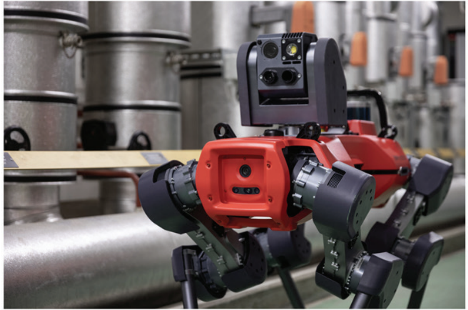
ANYmal's pan-tilt inspection unit features high-end sensors for accurate and reliable visual, thermal, and acoustic measurements.
