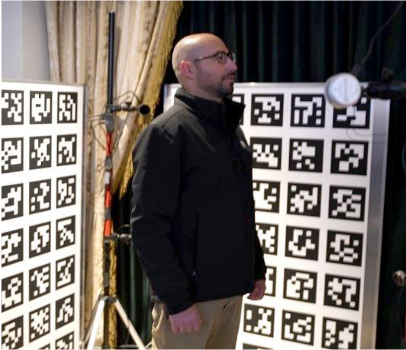
Figure 5. Flat targets containing optical fiducial markers were placed between the poles to facilitate alignment and extrinsic calibration of all the cameras.
