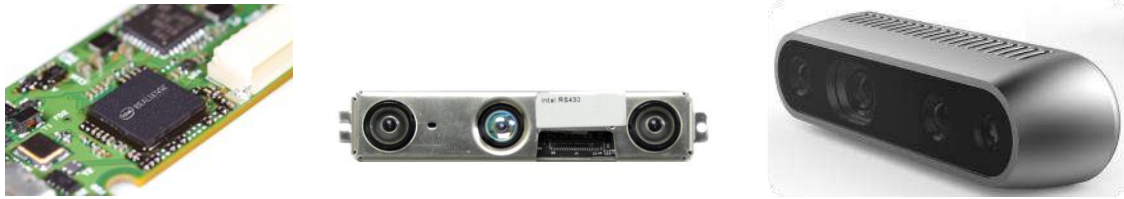
Fig. 7. Left: Intel RealSense™ D4m vision processor. Middle: Example of one of the Intel RealSense™ D4xx series depth modules encased in a steel case. RIGHT: Intel RealSense™ USB3 Depth Camera D435.
