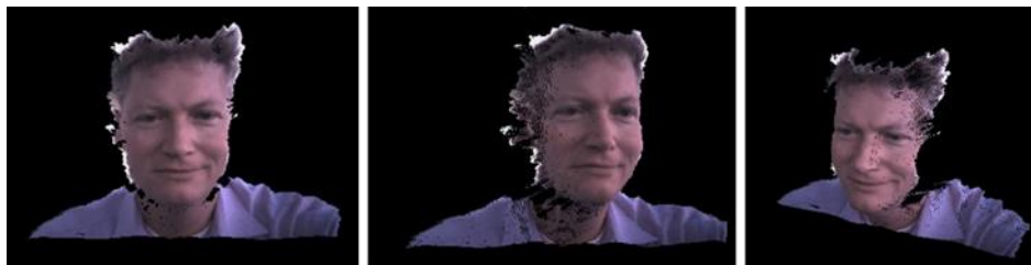
Fig. 3. A 3D-Selfie. The single photo was taken outside in full sunlight with a Depth Camera and is shown as a textured 3D point-cloud that is rotated to different views. Note that the true dimensions of the face are captured. In this picture anything beyond 0.6m was left out. For true Background Segmentation a more complex algorithm would be used that would yield cleaner edges and would use both RGB and Depth information.
