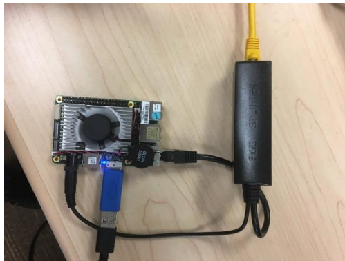
Figure 9. UP board being powered by PoE
