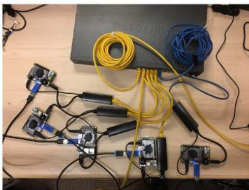
Figure 11. Ethernet server used with 5x UP Boards capturing depth from a Multiview RealSense cameras stage.
