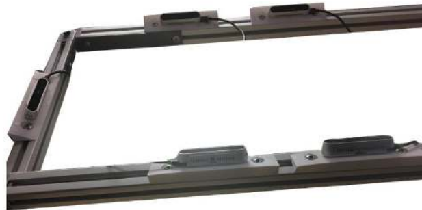
Figure 11. Ethernet server used with 5x UP Boards capturing depth from a Multiview RealSense cameras stage.
