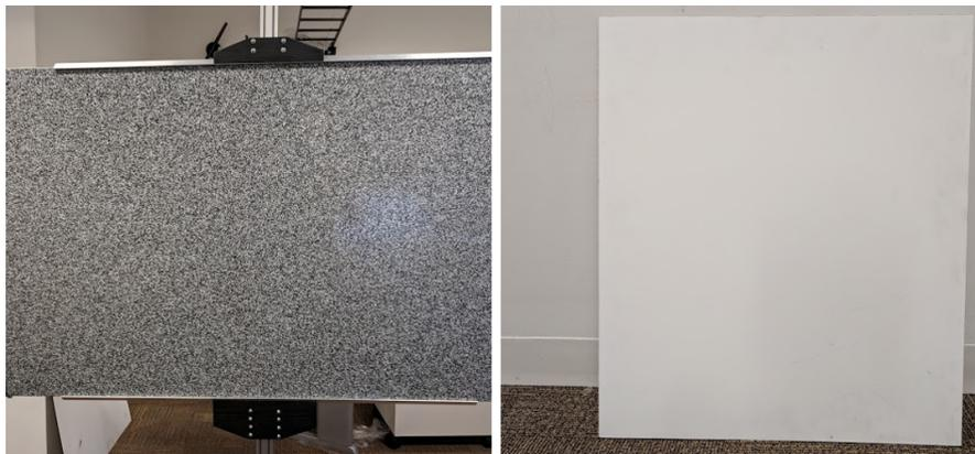
Fig. 13: Well-textured flat target (left) and white flat target (right).
