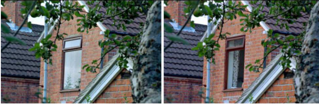
Figure 10. Photographs of a window with a polarizer filter rotated to two different angles. In the right picture, the polarizer was oriented to eliminate the strongly polarized reflected sunlight. Photographs reproduced from Ref. 6.
