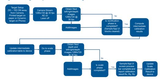
The advantage of targeted calibration is that it's accurate and consistent. It calibrates left/right depth as well as RGB (on devices with RGB). The disadvantage is that it
