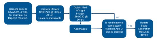
By default, target-less calibration supports 1280x720 resolution images. On devices with wide angle lenses such as D420, D430, D435, and D435i additional native resolution 1280x800 is also supported.
