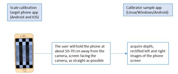
Figure 8-1 dynamic calibration simplified flow
