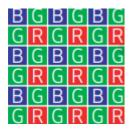
On devices with wide angle lens, for example, D420/D430/D435, the left and right imager sensors are monochrome. Demosaic is not needed.
