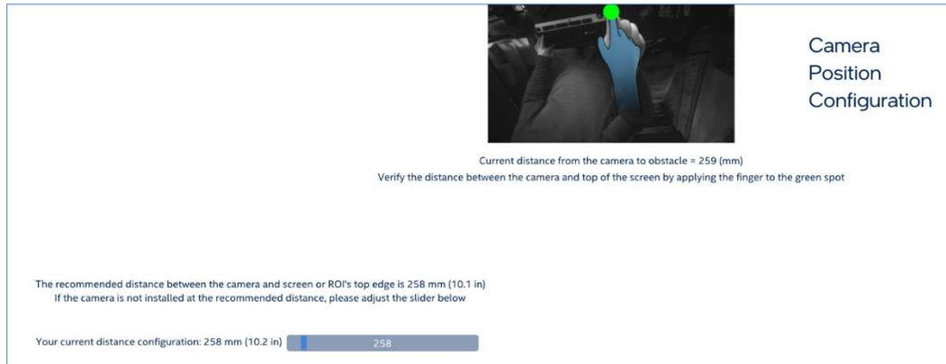
The tool display IR image so user can look through it to know if monitor is in the view. Rotate the camera forward until the monitor is not in the view.
