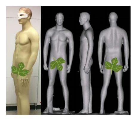
Figure 13. Example resultant 3D reconstruction derived from combining the point-clouds from the 8x L515 cameras
