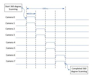
Figure 12. Example timing diagram of trigger signals sent to the 8 different L515 cameras used in the body scanning demonstration. Each camera (placed in slave mode), will only capture during signal-high. This diagram shows how pairs of cameras were turned on at a time, for 160ms captures, for a total capture time of 640ms.
