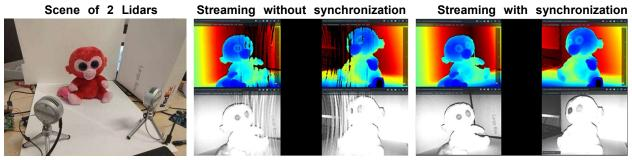
Figure 2: Examples of streaming simultaneously 2 Lidar in a high interference scenario where streams are not HW synchronized (middle image) showing stripe artifacts. The right-most image shows the case where interference has been eliminated (right) by using HW synchronization.
