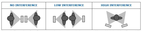
Figure 1: Examples of configurations showing objects being scanned by multiple Intel RealSense LiDAR Camera L515. By minimizing optical overlap, the system will be much less prone to interference, as shown by two images on left. However, the right most image shows two overlapping fields-of-view, which can lead to strong interference, unless properly mitigated.
