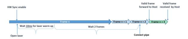
Figure 10. Enable received at least 10ms before end of frame
