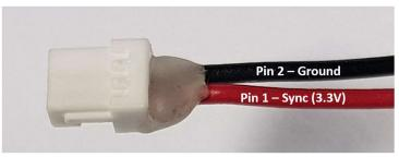
Figure 8. A close-up view of the connector and the connections. Pin 1 is the left-most pin as shown in the figure above. Pin 2 is the middle pin.
