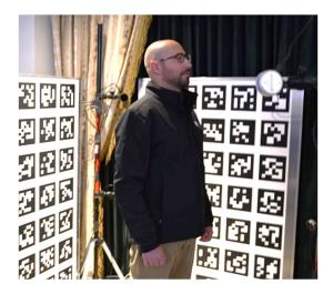
Figure 5. Flat targets containing optical fiducial markers were placed between the poles in order to facilitate alignment and extrinsic calibration of all the cameras.
