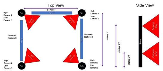
Figure 4. Body scanning camera configurations, corresponding to Figure 3, showing camera alignment in order to scan a human body. In this configuration, 8 cameras were used, as each pole had two cameras.
