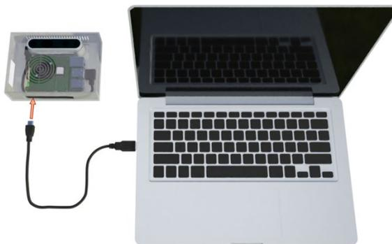
Figure 7. A PC can be directly connected to the Raspberry Pi via the USB3 type-C port
