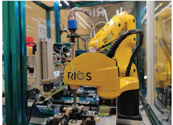
RIOS machine learning (ML) models utilize the data from Intel RealSense sensors to recognize the pose (orientation in space) and grasp points of objects in many different settings, enabling the robots to perform complex handling and manipulation such as picking and placing items into bins and moving them on and off of conveyor belts—two notoriously difficult examples of dynamic, ever shifting conditions.
